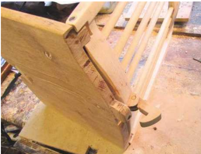
▲ Pic. 4 I was nervous about relying only on two blocks to hold the seat-back to the base, so reinforced it with a swivelling latch on the back, held by a small turnbuckle
